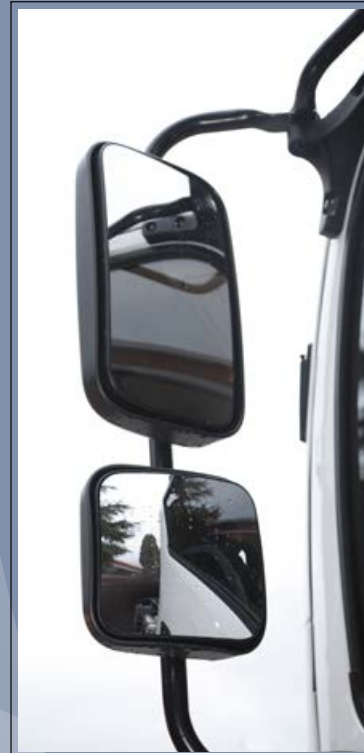
Electrically-operated and heated door mirrors
